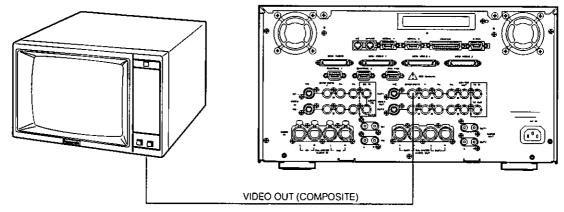
Coaxial Cable with BNC Connector
